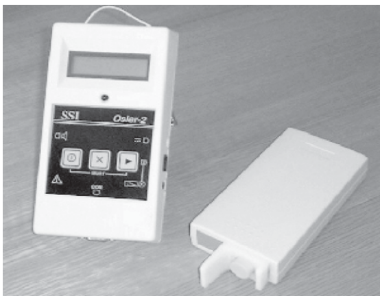
Fig. 7.2. OSleR test device: central unit, LED and LCD screen.
